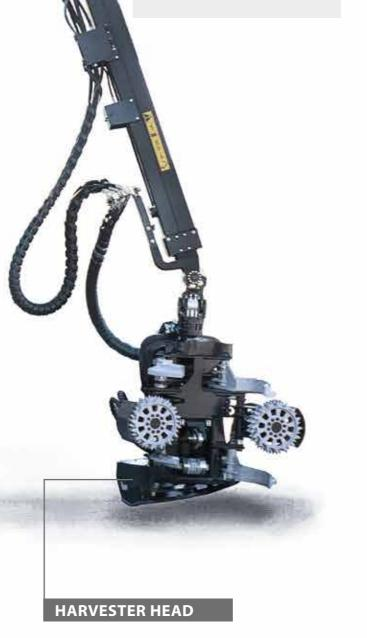
The Logset TH harvester head is key to higher productivity. The Logset 6HP GT can be equipped with a TH45, TH55 or TH65 harvester head, whichever size best meets the needs.
